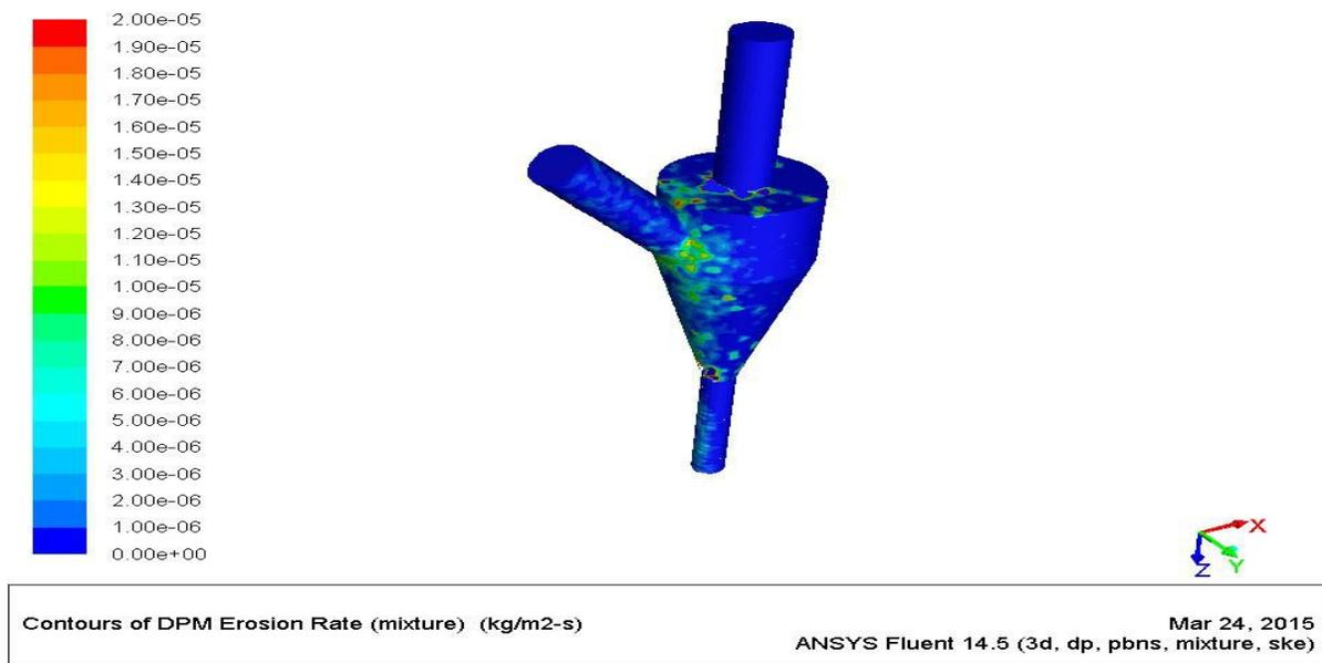
*Fig 4: contour of erosion rate for Aluminium oxide*
