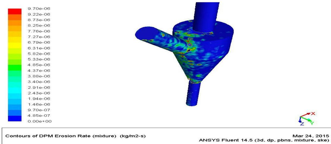
*Fig 10: Contour of erosion rate for tungsten carbide*
