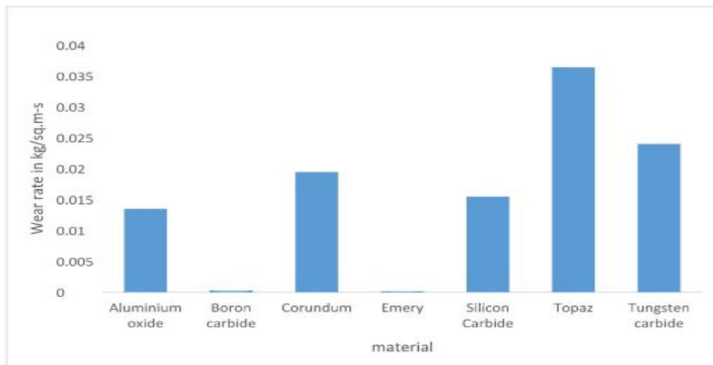
*Fig 11: Comparison of wear rates for various abrasives*
