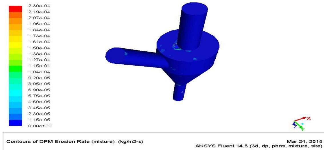
*Fig 5: contour of erosion rate for Boron Carbide*
