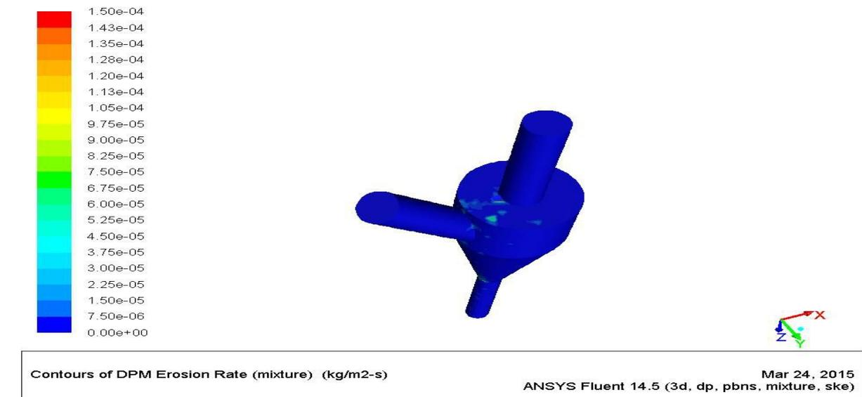
*Fig 7: Contour of erosion rate for Emery*
