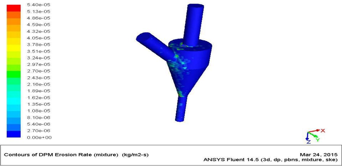
*Fig 9: Contour of erosion rate for topaz*
