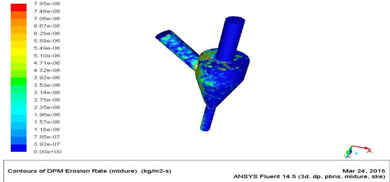
*Fig 6: Contour of erosion rate for Corundum*
