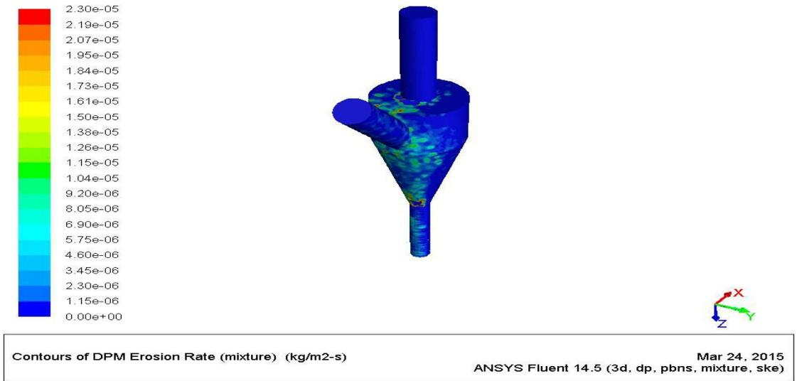
*Fig 8: Contour of erosion rate for Silicon Carbide*
